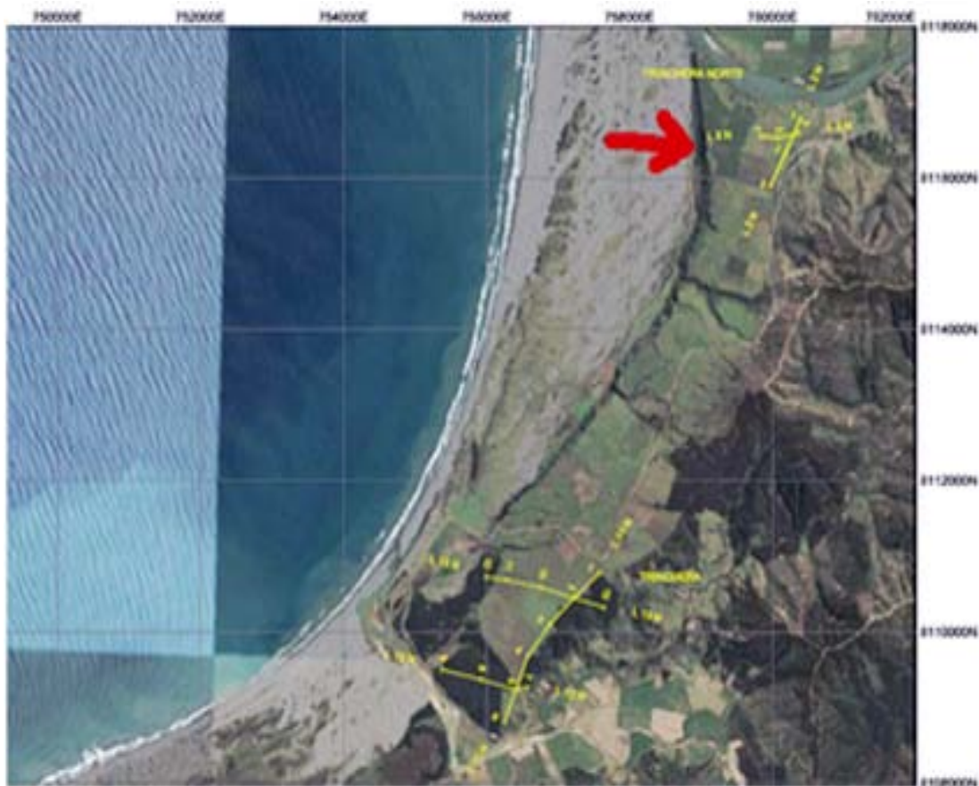
Fig. 7. Trincherá Prospect shown above in light green east of a dark line (arrowed) marking a cliff, and extending to the irregular dark green tones of older Paleozoic rocks. Yellow lines in the northern and southern sections of Trincherá are electrical resistivity survey lines.
